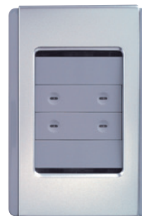
5854D1L2AA C-Bus Wireless Wall Switch, 4-Button, 2-Channel Leading Edge Dimmer, 250VA per Channel
